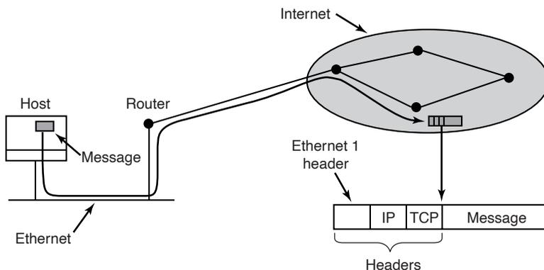
**Figure 8-31.** Accumulation of packet headers.
