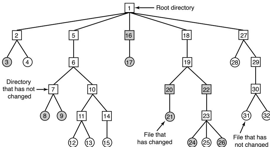
**Figure 4-27.** A file system to be dumped. The squares are directories and the circles are files. The shaded items have been modified since the last dump. Each directory and file is labeled by its i-node number.
