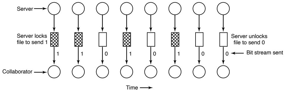
**Figure 9-24.** A covert channel using file locking.
