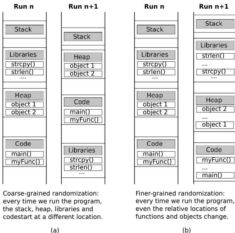
**Figure 9-33.** Address-space layout randomization: (a) coarse-grained (b) fine-grained
