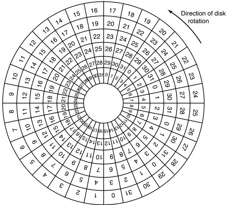
**Figure 5-20.** An illustration of cylinder skew.
