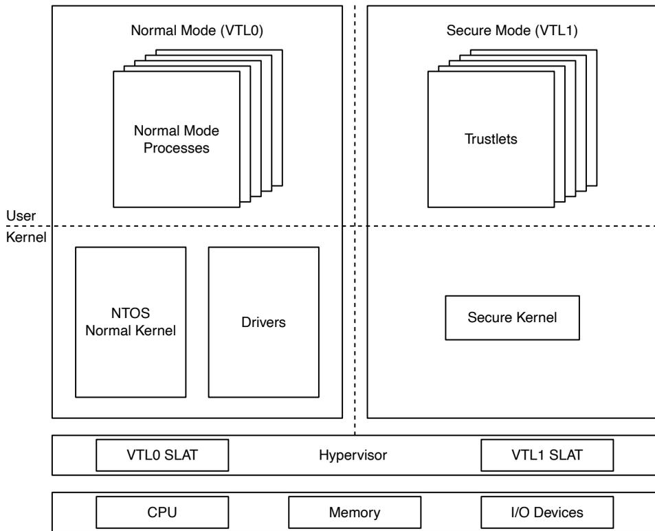
**Figure 11-54.** Virtual Secure Mode architecture with NT kernel in VTLO and Secure Kernel in VTL1. VTLs share memory, CPUs, and devices, but each VTL has its own access protections for these resources, controlled by higher VTLs.
