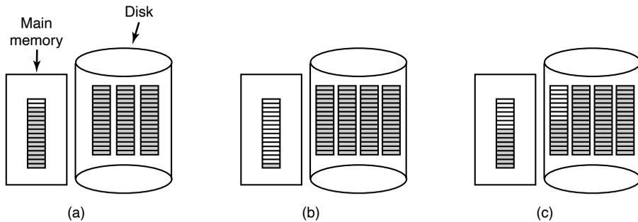
**Figure 4-25.** (a) An almost-full block of pointers to free disk blocks in memory and three blocks of pointers on disk. (b) Result of freeing a three-block file. (c) An alternative strategy for handling the three free blocks. The shaded entries represent pointers to free disk blocks.
