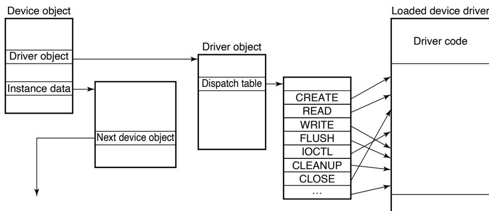
**Figure 11-41.** A single level in a device stack.
