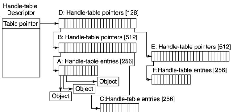
**Figure 11-17.** Handle-table data structures for a maximal table of up to 16 million handles.
