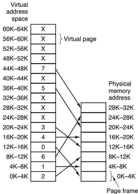
**Figure 3-9.** The relation between virtual addresses and physical memory addresses is given by the **page table**. Every page begins on a multiple of 4096 and ends 4095 addresses higher, so 4K-8K really means 4096-8191 and 8K-12K means 8192-12287.
