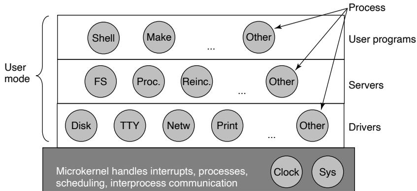
**Figure 1-26.** Simplified structure of the MINIX system.
