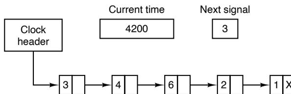
**Figure 5-29.** Simulating multiple timers with a single clock.
