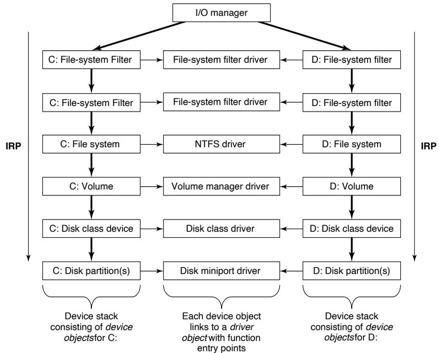
**Figure 11-14.** Simplified depiction of device stacks for two NTFS file volumes. The I/O request packet is passed from down the stack. The appropriate routines from the associated drivers are called at each level in the stack. The device stacks themselves consist of device objects allocated specifically to each stack.
