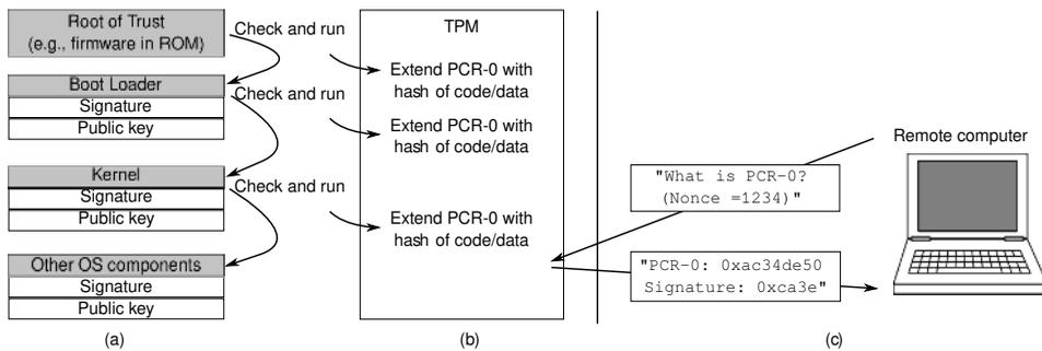
**Figure 9-35.** Securing and verifying the boot process.
