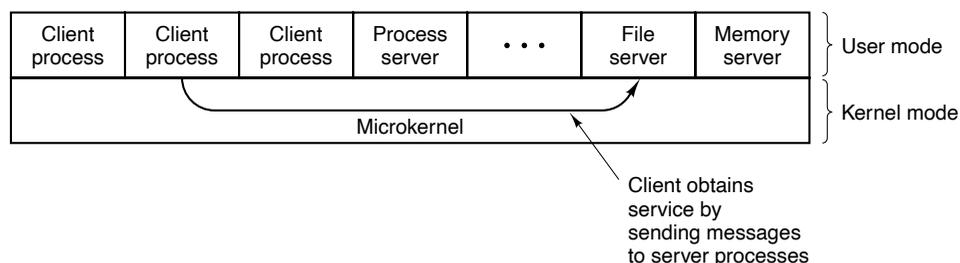
**Figure 12-3.** Client-server computing based on a microkernel.
