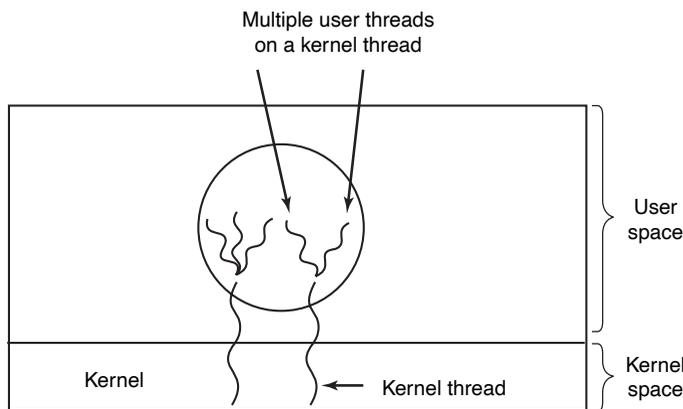
**Figure 2-16.** Multiplexing user-level threads onto kernel-level threads.
