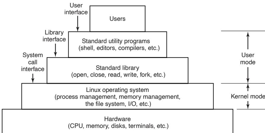
**Figure 10-1.** The layers in a Linux system.
