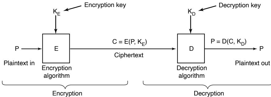
Figure 9-12. Relationship between the plaintext and the ciphertext.
