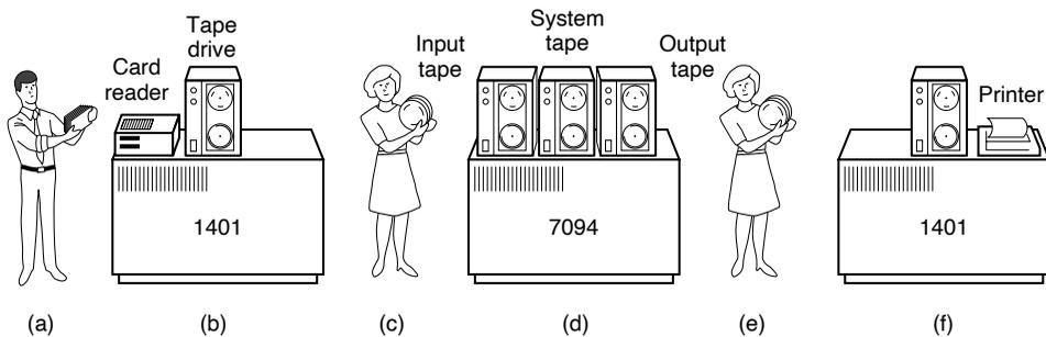
**Figure 1-3.** An early batch system. (a) Programmers bring cards to 1401. (b) 1401 reads batch of jobs onto tape. (c) Operator carries input tape to 7094. (d) 7094 does computing. (e) Operator carries output tape to 1401. (f) 1401 prints output.
