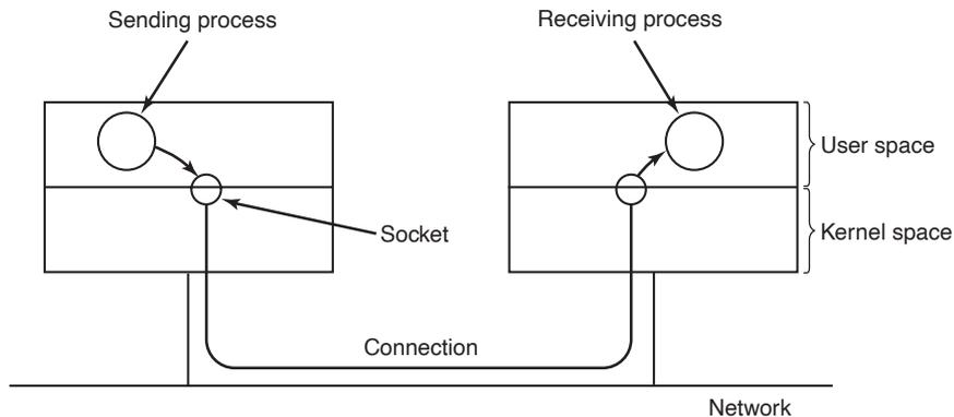
**Figure 10-19.** The uses of sockets for networking.
