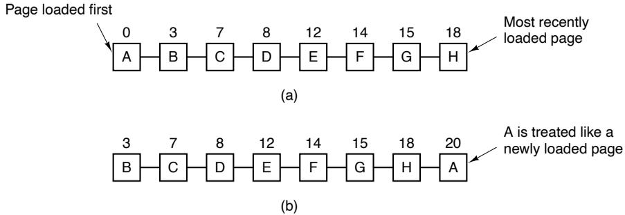
**Figure 3-15.** Operation of second chance. (a) Pages sorted in FIFO order. (b) Page list if a page fault occurs at time 20 and *A* has its *R* bit set. The numbers above the pages are their load times.
