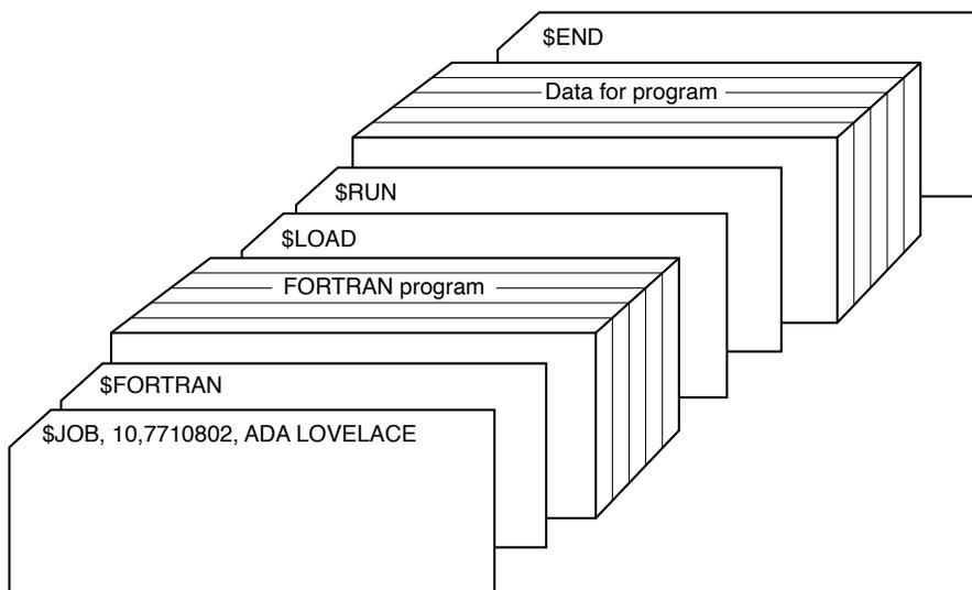
**Figure 1-4.** Structure of a typical FMS job.
