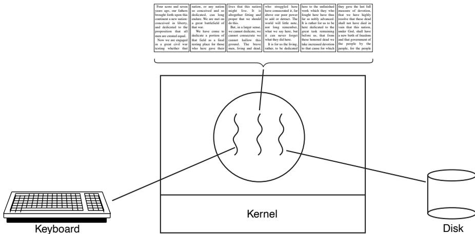
Figure 2-7. A word processor with three threads.
