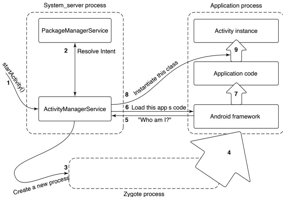
**Figure 10-62.** Steps in launching a new application process.
