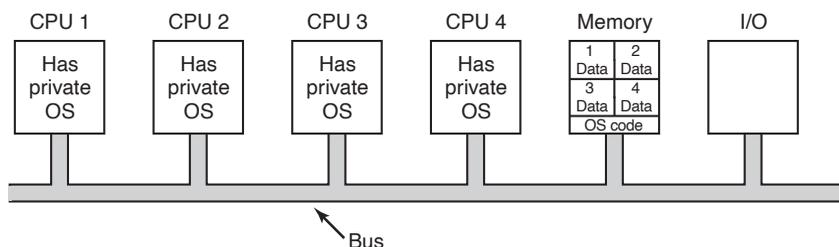
**Figure 8-7.** Partitioning multiprocessor memory among four CPUs, but sharing a single copy of the operating system code. The boxes marked Data are the operating system's private data for each CPU.
