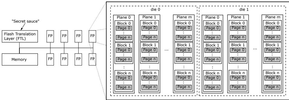
**Figure 4-20.** Components inside a typical flash SSD.
