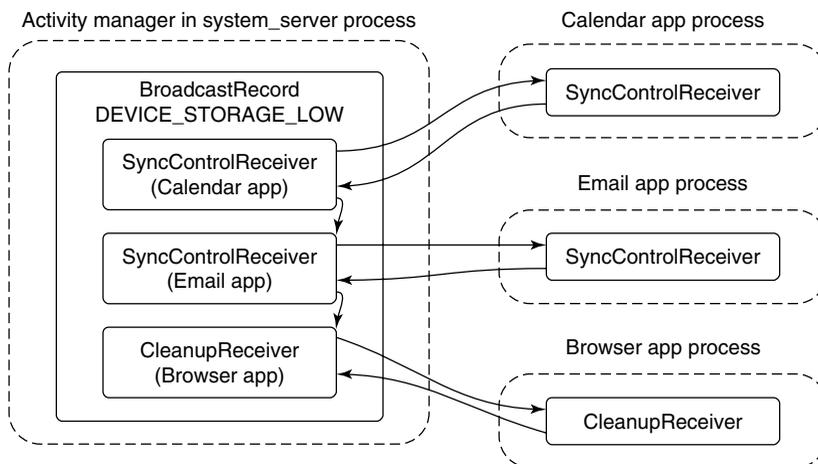
Figure 10-60. Sending a broadcast to application receivers.
