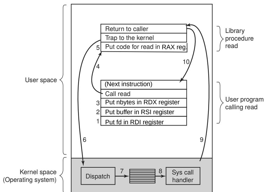
**Figure 1-17.** The 10 steps in making the system call `read(fd, buffer, nbytes)`.
