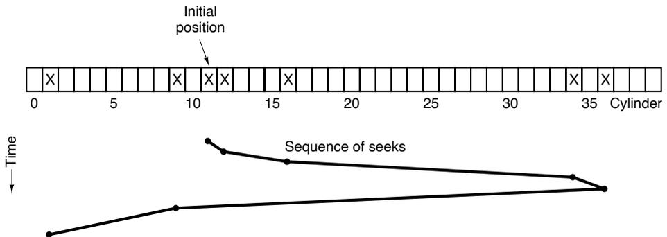
**Figure 5-23.** The elevator algorithm for scheduling disk requests.
