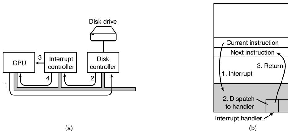
**Figure 1-11.** (a) The steps in starting an I/O device and getting an interrupt. (b) Interrupt processing involves taking the interrupt, running the interrupt handler, and returning to the user program.
