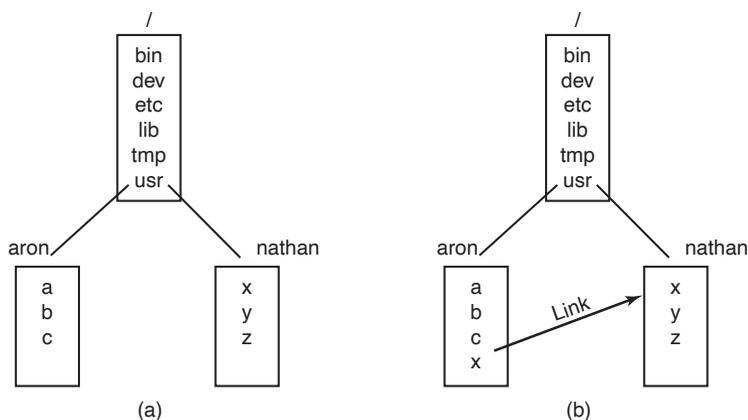
**Figure 10-24.** (a) Before linking. (b) After linking.
