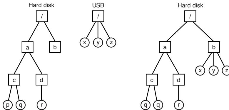
**Figure 10-25.** (a) Separate file systems. (b) After mounting.
