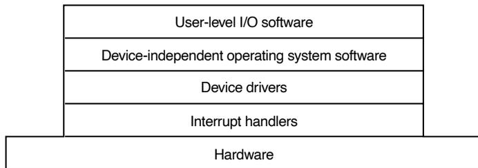
**Figure 5-11.** Layers of the I/O software system.
