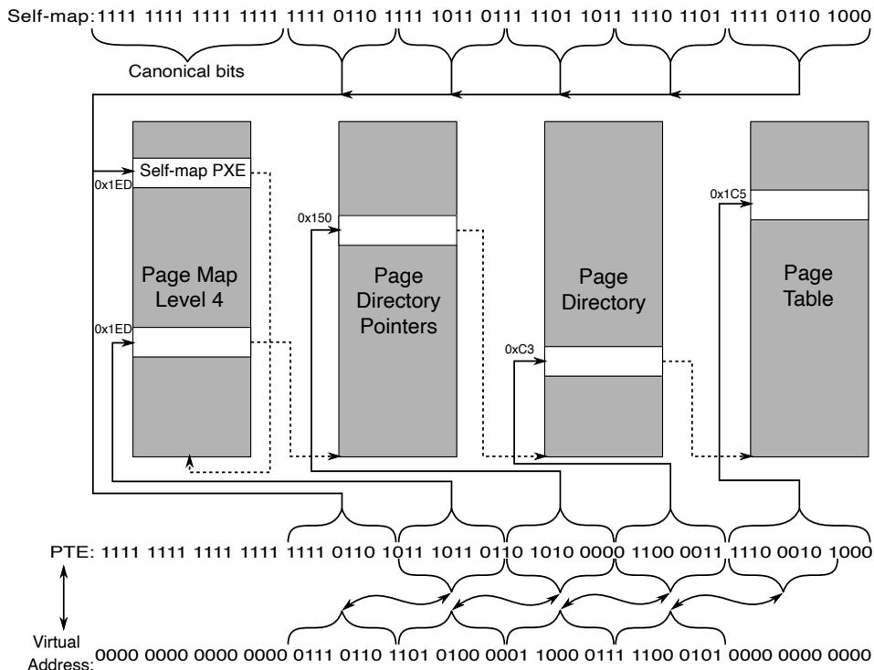
**Figure 11-35.** The Windows self-map entries are used to map the physical pages of the page table hierarchy into kernel virtual addresses. This makes conversion between a virtual address and its PTE address very easy.
