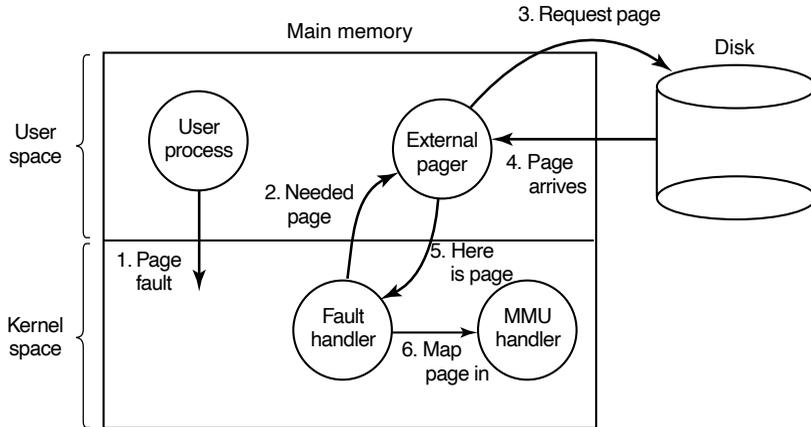
**Figure 3-29.** Page fault handling with an external pager.
