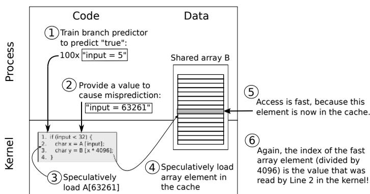
**Figure 9-30.** Original Spectre attack on the kernel.
