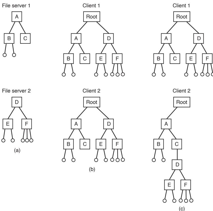
**Figure 8-34.** (a) Two file servers. The squares are directories and the circles are files. (b) A system in which all clients have the same view of the file system. (c) A system in which different clients have different views of the file system.
