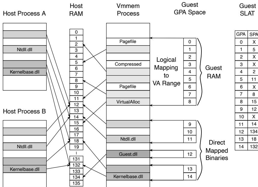
**Figure 11-52.** VA-backed VM's GPA space is logically mapped to virtual address ranges in its vmmem process on the host.
