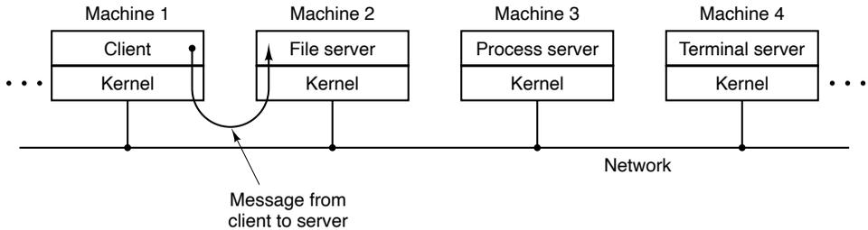
**Figure 1-27.** The client-server model over a network.
