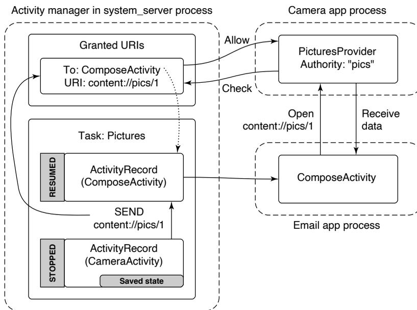
**Figure 10-69.** Sharing a picture using a content provider.
