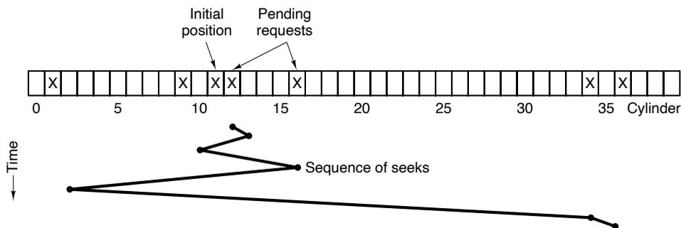
**Figure 5-22.** Shortest Seek First (SSF) disk scheduling algorithm.
