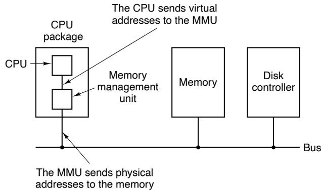
**Figure 3-8.** The position and function of the MMU. Here the MMU is shown as being a part of the CPU chip because it commonly is nowadays. However, logically it could be a separate chip and was years ago.
