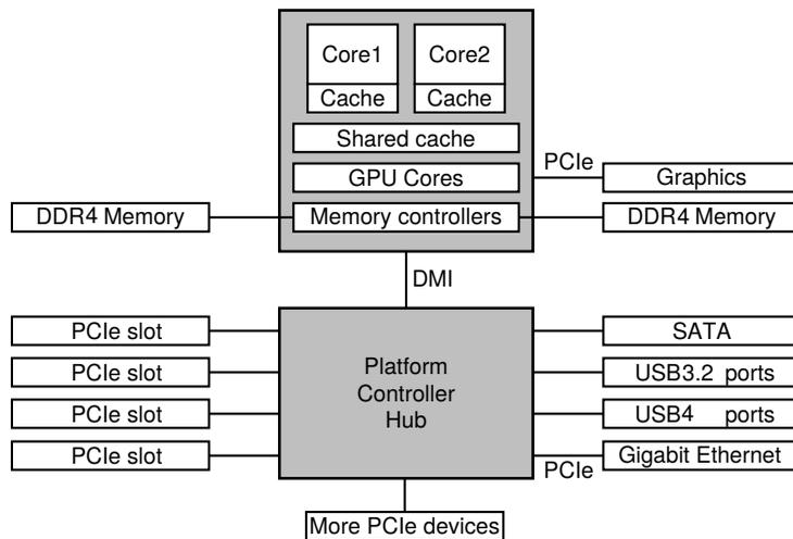
**Figure 1-12.** The structure of a large x86 system.
