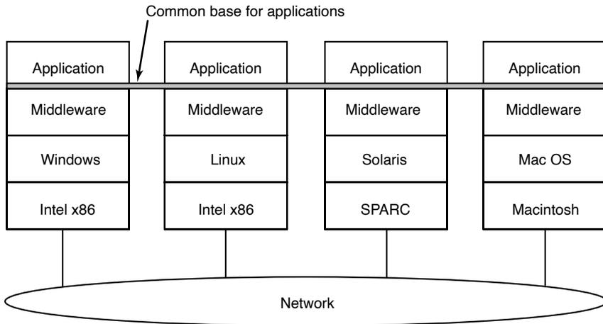
**Figure 8-27.** Positioning of middleware in a distributed system.
